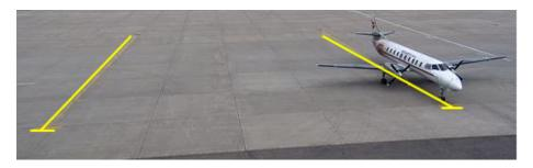
T-lines are located on Apron II only at this time. There are two located in the Restricted Area of the Apron, and four in the Controlled Area of the Apron. Remember that the Restricted Area is used to park aircraft for embarking and disembarking passengers; which includes additional security considerations.
